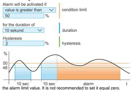
Thus, the setting for generating an alarm is completed. It remains to decide, whether the alarm should be indicated optically by means of a LED diode on the device (*Optical signalling - LED*), acoustically (*Activate internal acoustic signalling*) or by sending a alarm text message to up to four selected recipients (when alarm occurs/disappears, send SMS to selected recipients).
