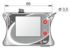
You can fix the device on the wall with the aid of a lockable holder
